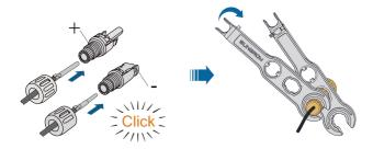
step 4 Check for polarity correctness.
